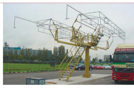
KANON's Loading Platforms are used worldwide to achieve safe and easy top access of road and rail tankers from ground level. The Loading Platforms, combined with loading equipment, offer a complete solution without need for separate
