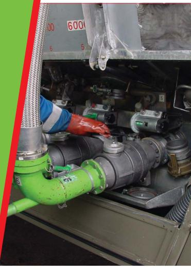
KANON cross-over bottom loading arms allow simultaneous connecting and filling of up to seven product lines with vapour return.
