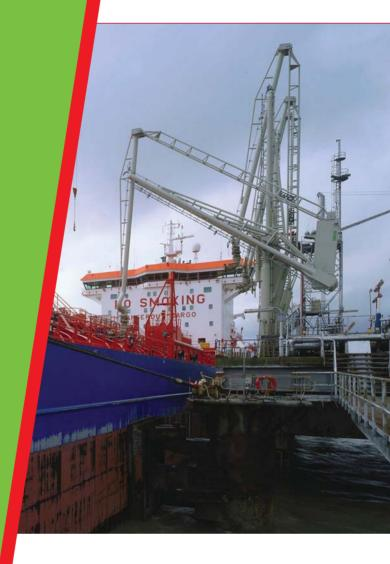
The transfer of all fluids and liquefied gases, into the smallest barge or the largest crude carrier may be safely and dependably accomplished using a KANON Marine Loading Arm system.
