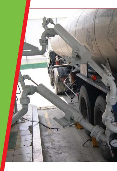
The advantage of Bottom Loading Arms is that these can be operated at ground level without need for loading platforms.
